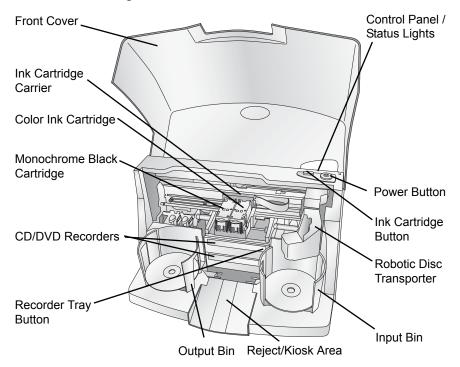
The **Robotic Disc Transporter** moves discs from the Input Bin, to a CD/DVD Recorder, to the printer, and finally to the Output Bin.
